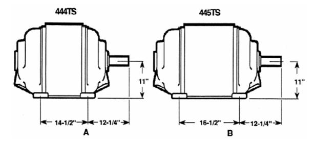
The length difference in the examples above occurs between the feet as shown by dimensions A and B. The suffix T indicates that the motor frame assignment conforms to the current, or so called "T" frame "Nu-Rate" standards which were adopted in 1964.
